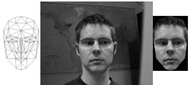
Figure 2: A generic 3D polygonal head model is aligned with a head-on shot of the video sequence, and the corresponding pixels are texture mapped to the surface of the face model.
