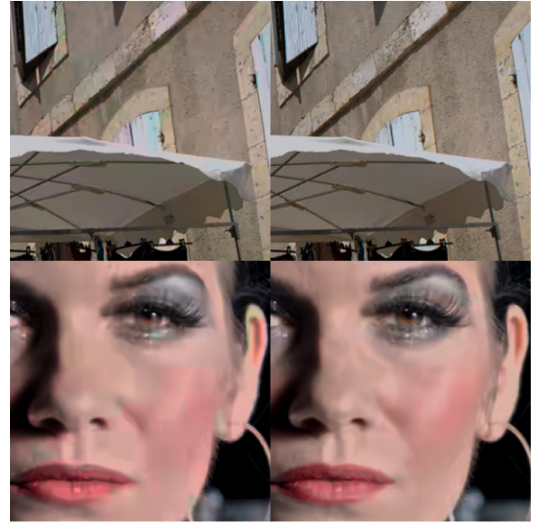
Fig. 2. Left column: Traditional processing (MPEG CfE Anchor). Right column: Proposed method, Anchor 3.2 in MPEG/JCT-VC at a similar but lower bit rate. Note how the color artifacts that are present on the left are ameliorated on the right. Texture is also more detailed. Top sequence courtesy of Technicolor and the NevEx project.
