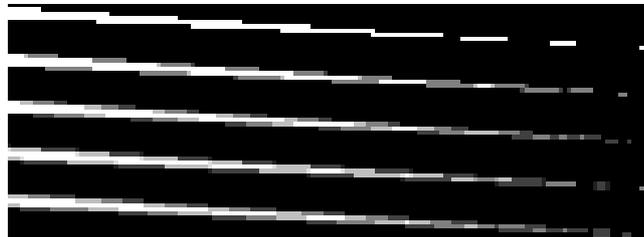
Figure 9: Evaluation of sampling schemes for thin features. From top to bottom: one sample per pixel,  $2 \times 2$  samples (brute force), RGSS, Quincunx, and FLIPQUAD.
