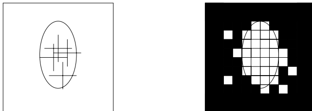
Figure 1: Left: Output of an algorithm that tries to find the center of the face (the ellipse). Right: Our algorithm lets each block of pixels determine whether it is part of the face or not.
