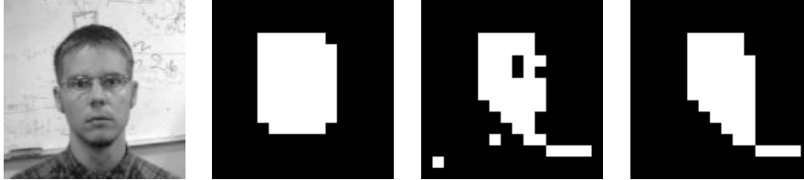
Figure 4: From left: Original image (not in training sequence), true face-map, network output and final result after cleaning. Error rate = 11%.
