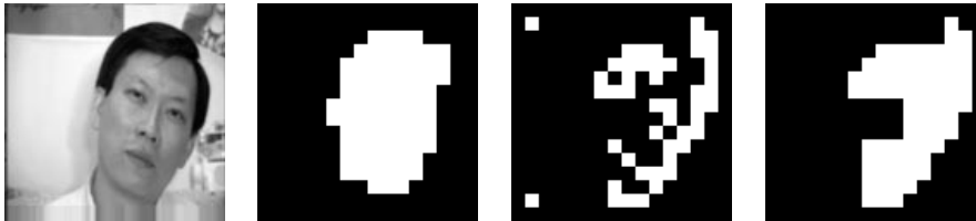
Figure 5: From left: Original image (not in training sequence), true face-map, network output and final result after cleaning. Note the big impact of the cleaning filter, from 35% errors to 20%.
