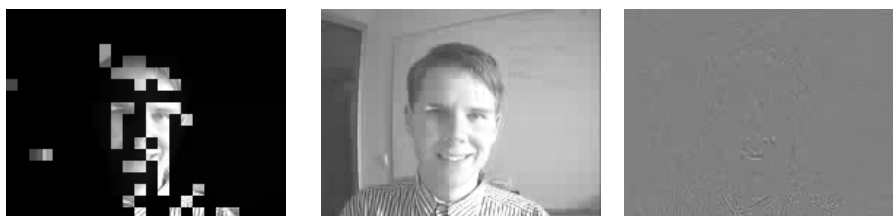
Figure 11: Blocks selected by the DC thresholding algorithm. Figure 12: 2nd image using DC thresholding, 1052 bytes. Figure 13: Error introduced by DC thresholding.
