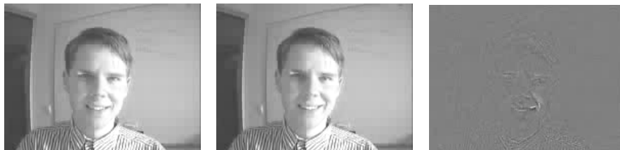
Figure 8: First image in the sequence. Figure 9: Second image, 5538 bytes. Figure 10: Difference between 1st and 2nd.
