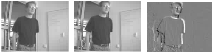
Figure 14: First image in the sequence. Figure 15: Second image, 5646 bytes. Figure 16: Difference between 1st and 2nd.
