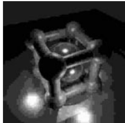
Figure 19: Wavelet decompressed picture. Compression ratio 63.7. File length 4114 bytes. Figure 20: JPEG decompressed picture. Compression ratio 60.5. File length 4334 bytes.
