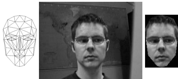
Fig. 8. A generic three-dimensional polygonal head model is aligned with a head-on shot of the video sequence, and the corresponding pixels are texture mapped to the surface of the face model.
